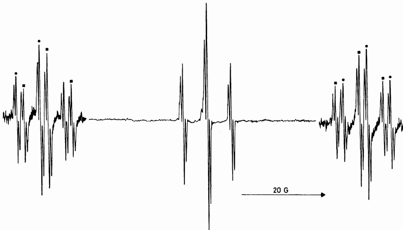
FIGURE 1 E.s.r. spectrum of the trimethyltin radical adduct with bis-2-thieno[2,3- b ]thienyl ketone (IV). The satellite lines due to ^{117}\text{Sn} (■) and ^{119}\text{Sn} (●) have been recorded with higher amplification
